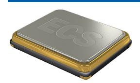
ECS Inc's CDX-1932 is a 39 MHz SMD Crystal offered in a 2.00 mm x 1.60 mm x 0.45 mm, 4-pad industry standard package. Features include a 10pF load capacitance, a 35 $\Omega$  ESR, and is available in 1,000-piece or 3,000-piece reel option (-TR3).
