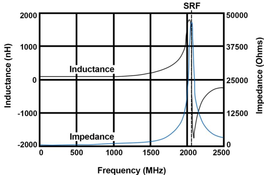
Figure 1 illustrates the apparent inductance as measured by a LCR meter. An LCR meter is a type of electronic test equipment to measure the inductance (L), capacitance (C), and resistance (R) of an electronic component.
